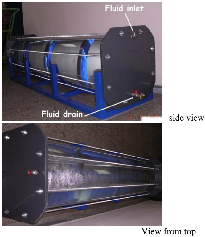
Figure 4: Simulator for the agents testing in a static fluidic environment
